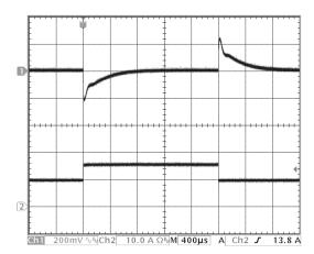
Figure 12: Output voltage response to step-change in load current (50%-75%-50% of Iout(max):  $dI/dt = 5A/\mu s$ ). Load cap:  $470\mu F$ , 30 m $\Omega$  ESR tantalum capacitor and 1µF ceramic cap. Ch 1: Vout (200mV/div), Ch 2: Iout (10A/div).
