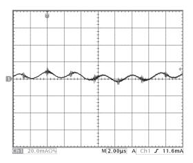
Figure 15: Input reflected ripple current,  $i_s$  through a 3.3  $\mu$ H source inductor at nominal input voltage and rated load current (20 mA/div). See Figure 13.
