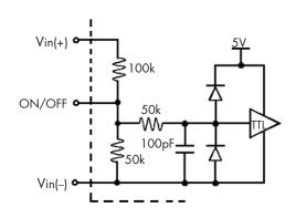
Figure B: Internal ON/OFF pin circuitry
