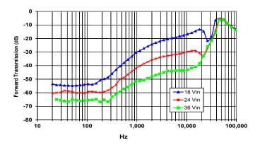
Figure 20: Magnitude of incremental forward transmission (FT =  $v_{out}/v_{in}$ ) for minimum, nominal, and maximum input voltage at full rated power.
