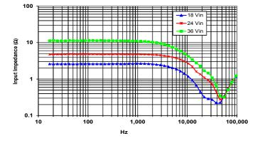
Figure 22: Magnitude of incremental input impedance  $(Z_{in} = v_{in}/i_{in})$  for minimum, nominal, and maximum input voltage at full rated power.
