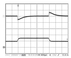
Figure 11:Output voltage response to step-change in load current (50%-75%-50% of Iout(max);  $dI/dt = 0.1A/\mu s$ ). Load cap:  $10\mu F$ ,  $100 \text{ m}\Omega$  ESR tantalum capacitor and 1µF ceramic capacitor. Ch 1: Vout (200mV/div), Ch 2: Iout (10A/
