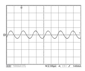
Figure 14: Input Terminal Ripple Current,  $i_e$  at full rated output current and nominal input voltage with 3.3 $\mu$ H source impedance and  $100\mu$ F electrolytic capacitor (500 mA/div). See Figure 13.
