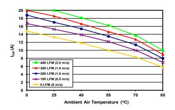
Figure 7: Maximum output power-derating curves vs. ambient air temperature for airflow rates of 0 LFM through 400 LFM with air flowing from input to output (nominal input voltage).
