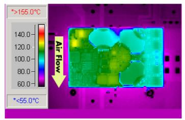
Figure 6: Thermal plot of converter at 14 amp load current (70W) with 55°C air flowing at the rate of 200 LFM. Air is flowing across the converter from pin 1 to pin 3 (nominal input voltage).
