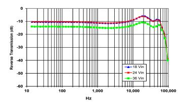
Figure 21: Magnitude of incremental reverse transmission (RT =  $i_{in}/i_{out}$ ) for minimum, nominal, and maximum input voltage at full rated power.
