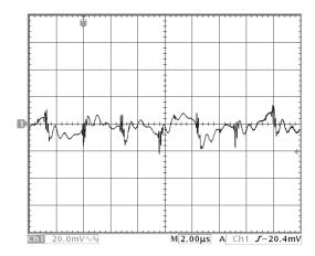
Figure 16: Output voltage ripple at nominal input voltage and rated load current (20 mV/div). Load capacitance: 1μF ceramic capacitor and 10μF tantalum capacitor. Bandwidth: 20 MHz. See Figure 13.
