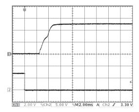
Figure 10: Turn-on transient at zero load (2 ms/div). Ch 1: Vout (2V/div) Ch 2: ON/OFF input (5V/div)
