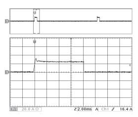
Figure 18: Load current (20A/div) as a function of time when the converter attempts to turn on into a 10 m $\Omega$  short circuit. Top trace (2.5ms/div) is an expansion of the on-time portion of the bottom trace.
