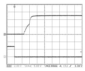
Figure 9: Turn-on transient at full load (resistive load) (2 ms/div). Input voltage pre-applied. Ch 1: Vout (2V/div). Ch 2: ON/OFF input (5V/div)
